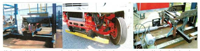
If a heavy vehicle have an energy-absorbing front, rear and side under-run protection it could reduce deaths in car by about 12%. In EU it is mandatory for vehicles over 3.5 tonnes to have a rigid front underrun protection system.
