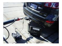
The testing required for towbars is straight forward and can be preformed by a company specialising in material testing using a portable hydraulic power unit. Something that ASE has two of, this make the testing of towbar more efficient and give you a faster turnover time. ASE also do two types of tests, a static test and a cycle test to make sure we cover all parts on how to test a towbar.
